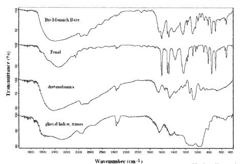
Fig.1. IR Spectrum of bis-Mannich base polyol on phenol based, as acid substrat compared with IR spectrum of raw materials
